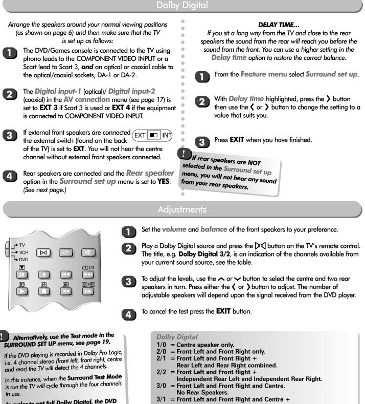
In order to get full Dolby Digital, the DVD player must be connected using the coaxial or optical links.
